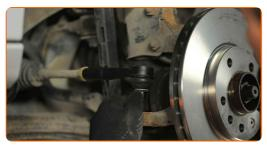
Tighten the fastening nut connecting the tie rod end to the steering knuckle. Use a drive socket #18. Use a torque wrench. Tighten it to 30 Nm torque.+90°
