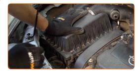
Screw in the fastening screws of the air filter cover. Use Torx T25.
