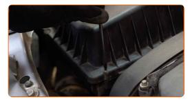
Unplug the mass air flow sensor connector.
