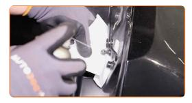
Install the new boot lid gas strut.
