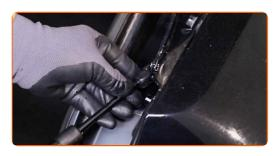
Snap on the circlip connecting the gas strut to the boot lid.
