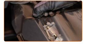
Unscrew the fasteners of the passenger side kick panel.
