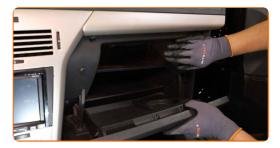
Screw the glove box fastening screws. Use Torx T20.
