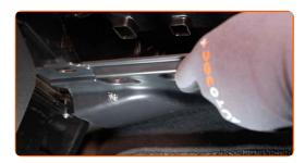
Unscrew the fasteners of the cabin filter housing cover. Use a drive socket #5.5. Use a ratchet wrench.
