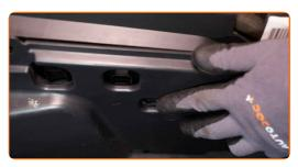
Screw in the fasteners of the passenger side kick panel.
