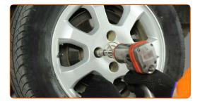
Lower the car and working in a cross order, tighten the wheel bolts. Use wheel impact socket #17. Use a torque wrench. Tighten it to 110 Nm torque.
