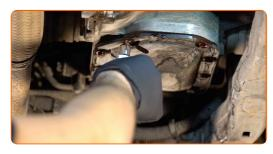
10 Remove the transmission fluid pan.
