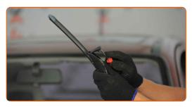
Remove the blade from the wiper arm.
