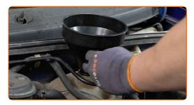
Pour coolant in the coolant reservoir.
