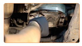
10 Remove the transmission fluid pan.
