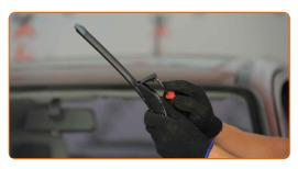
Remove the blade from the wiper arm.
