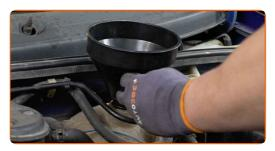
Pour coolant in the coolant reservoir.
