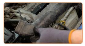
Clean the coolant hose connections. Use all-purpose cleaning spray.
