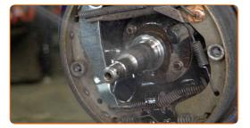
24 Install the brake drum assembled with the wheel hub bearing.
