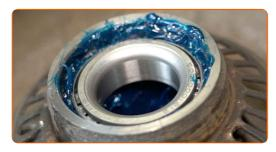
Install the wheel bearing oil seal.
