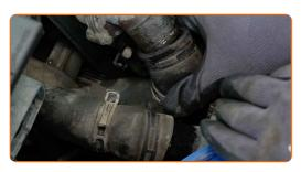
Replacement: engine thermostat – OPEL ASCONA B (81\_, 86\_, 87\_, 88\_). AUTODOC recommends:
