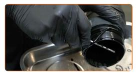
Clean the oil filter housing cap. Use all-purpose cleaning spray.
