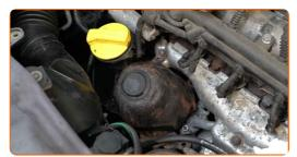
Screw in the fasteners of the protective case of the oil filter housing. Use Torx T25. Use a drive socket #10. Use a ratchet wrench.
