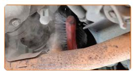
Detach the oxygen sensor connector.
