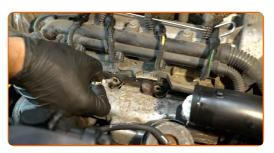
Tighten the glow plugs. Use the spark plug socket #8. Use a torque wrench. Tighten it to 10 nm torque.
