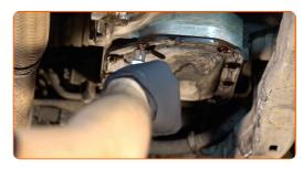
10 Remove the transmission fluid pan.
