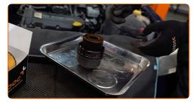
Cover the oil filter housing with a microfibre towel to prevent dirt and foreign objects from getting into the system.
