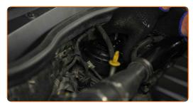
16 Attach the pipe to the fuel filter.
