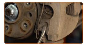
11 Remove the brake caliper.
