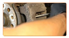
Remove the brake caliper. Use a crowbar.
