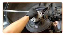
19 Remove the fastening bolt.
