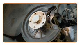
27 Install the brake disc.
