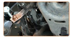
Remove the caliper bracket.
