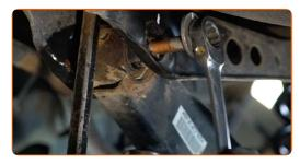
Adjust the position of the alignment bolt according to the mark.
