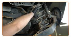
Remove the rubber spring spacer.
