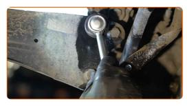
Tighten the stabiliser link fastener. Use a combination spanner #16. Use a drive socket #16. Use a ratchet wrench.
