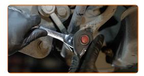
Unscrew the fastener connecting the stabilizer bar with the control arm. Use a combination spanner #16.
