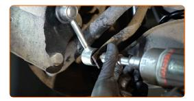
Tighten the fastener connecting the stabilizer bar with the control arm. Use a drive socket #16. Use a torque wrench. Tighten it to 45 Nm torque.
