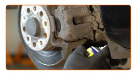
Unscrew the brake caliper fastening. Use a combination spanner #13. Use a combination spanner #15.
