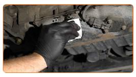
Screw in the new drainage plug and tighten it. Use a drive socket #19. Use a torque wrench. Tighten it to 26 Nm torque.
