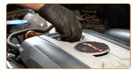
Tighten the oil filler cap.
