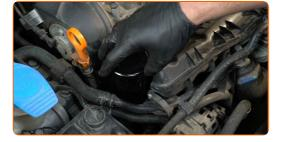
Screw the new filter into its place. Use the 77/15-F socket. Use a torque wrench. Tighten it to 24 Nm torque.
