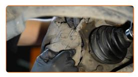
20 Install the brake caliper retaining spring.
