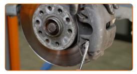
11 Remove the brake caliper.
