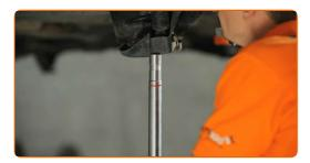
Tighten the lower fastener of the shock absorber. Use a combination spanner #16. Use a drive socket #16. Use a torque wrench. Tighten it to 40 Nm torque.+90°
