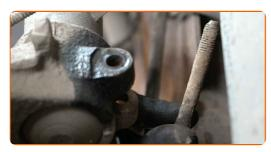
Disconnect the steering knuckle from the shock absorber strut. Use a rubber mallet.
