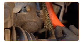
Unscrew the lower fastener connecting the shock strut to the steering knuckle. Use a combination spanner #18. Use a drive socket #18. Use a ratchet wrench.
