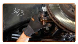
Tighten the fastening nut connecting the tie rod end to the steering knuckle. Use a drive socket #19. Use a torque wrench. Tighten it to 45 nm torque.
