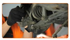
Disconnect the ball joint from the steering knuckle. Use a ball joint puller.
