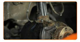
Connect the ABS sensor wiring.
