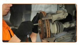
54.1 Install the brake caliper and fix it.
