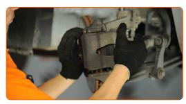
Use HEX No.H7. Use a torque wrench. Tighten it to 28 Nm torque.
