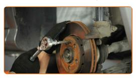
Remove the brake disc. Use a rubber mallet.
