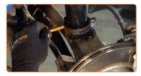
Tighten the lower fasteners of the suspension strut. Use a combination spanner #18. Use a drive socket #18. Use 40 a torque wrench. Tighten it to 60 Nm torque.+90°  $\,$
