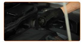
Tighten the oil filler cap.
