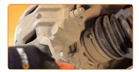
Unscrew the brake caliper fastening. Use a combination spanner #17. Use a drive socket #14. Use a ratchet wrench.
