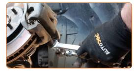
9 Remove the brake caliper.
