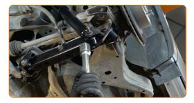
Replacement: rear suspension lower control arm - NISSAN X-Trail (T32). Tip:
