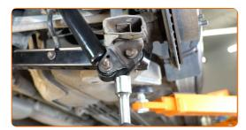
Tighten the fastener connecting the suspension arm to the rear knuckle. Use a combination spanner #18. Use a drive socket #21. Use a torque wrench. Tighten it to 150 Nm torque.
