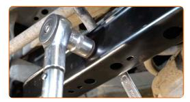
Remove the support from under the arm.
