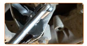
Unscrew the fastener connecting the control arm to the rear knuckle. Use a combination spanner #18. Use a drive socket #21. Use a ratchet wrench.
