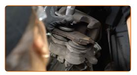
Install the brake caliper and fix it. Use a combination spanner #17. Use a drive socket #14. Use a torque wrench. Tighten it to 34 Nm torque.
