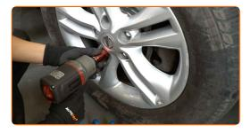
Lower the car and working in a cross order, tighten the wheel bolts. Use wheel impact socket #21. Use a torque wrench. Tighten it to 112 Nm torque.
