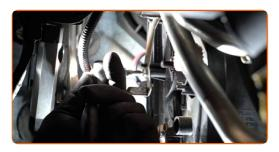
18 Install the heater flap actuator.
