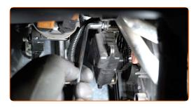
Remove the heater flap actuator.
