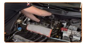
Plug in the ignition coil connector.
