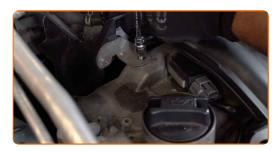
Attach the vacuum booster hose to the intake manifold.
