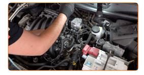
Connect the crankcase ventilation hose to the air duct. Use round-nose pliers.
