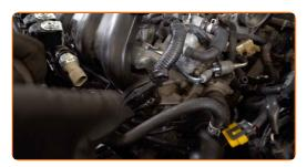
11 Remove the intake manifold.
