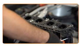
Remove the intake manifold gasket. Use a flat screwdriver.
