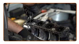
23 Install the new intake manifold gasket.
