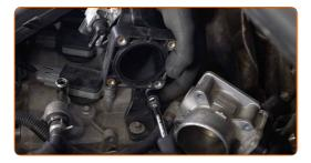
Detach the vacuum booster hose from the intake manifold.
