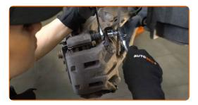
10 Remove the brake caliper.
