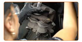
Install the brake caliper and fix it. Use a combination spanner #17. Use a drive socket #14. Use a torque wrench. Tighten it to 34 Nm torque.
