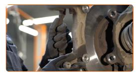
15 Remove the brake disc.
