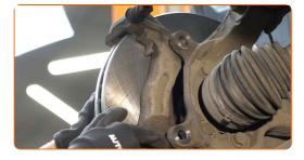
Tighten the brake caliper bracket. Use a drive socket #19. Use a torque wrench. Tighten it to 152 Nm torque.
