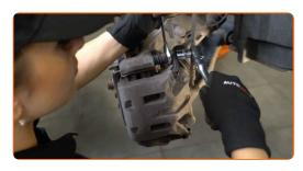
10 Remove the brake caliper.
