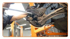
Remove the caliper bracket.
