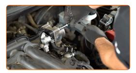
Release the clamp and detach the connector and the vacuum hose from the intake manifold near the throttle valve. Use round-nose pliers.
