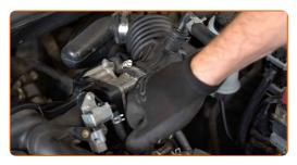
Unscrew the clamps and fasteners on the air filter intake pipe. Use a drive socket #10. Use a ratchet wrench.
