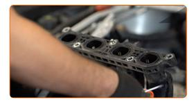
Remove the intake manifold gasket. Use a flat screwdriver.
