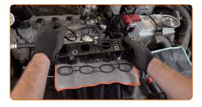
24 Install the intake manifold.
