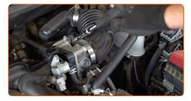
5 Disconnect the air intake pipe from the air filter housing.
