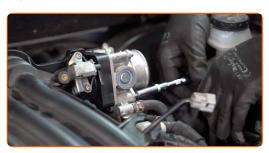
Attach the connector and the vacuum hose to the intake manifold near the throttle valve. Use round-nose pliers.
