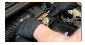
Reinstall the air filter cover. Fasten it.
