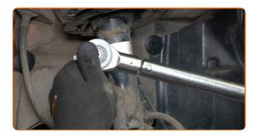
Tighten the fastener connecting the stabilizer link to the stabilizer bar. Use a drive socket #17. Use a torque wrench. Tighten it to 44 Nm torque.
