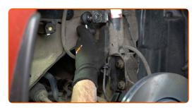
Tighten the fastener connecting the stabilizer link to the shock strut. Use a drive socket #17. Use a torque wrench. Tighten it to 44 Nm torque.
