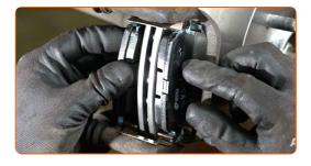
Clean the brake caliper guide pins. Use a brake cleaner.
