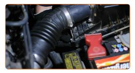
Unscrew the fuel filter bracket fixing bolts. Use a drive socket #10. Use a ratchet wrench. Use a Phillips screwdriver.
