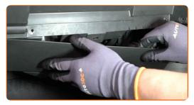
Remove the rear panel of the glove box.
