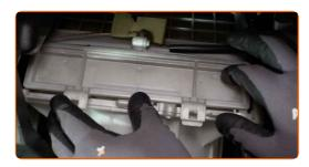
Attach the fasteners connecting the relay to the rear panel.
