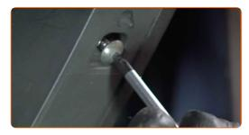
Detach the fasteners connecting the relay to the rear panel. Use pliers.
