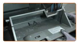
Unscrew the fasteners on the rear panel of the glove box. Use Torx T20.
