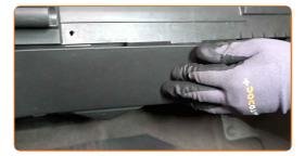
Screw in the fasteners on the rear panel of the glove box. Use Torx T20.
