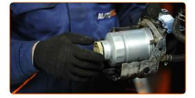
Install the new fuel filter together with its bracket.
