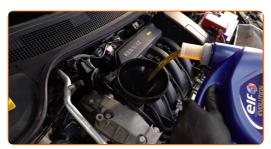
Replacement: engine oil and filter – NISSAN Sunny III Hatchback (N14). Tip:
