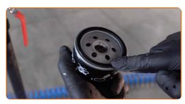
Screw the new filter into its place. Use the 76/14-F socket. Use a torque wrench. Tighten it to 21 nm torque.
