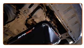
Unscrew the drain plug. Use square oil drain plug socket No.8 Use a ratchet wrench.
