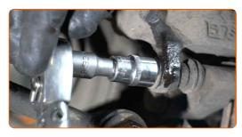
9 Remove the brake caliper guide pins.
