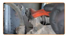
Unscrew the brake caliper fasteners. Use a drive socket #14. Use a ratchet wrench.
