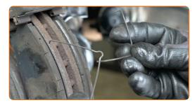
Remove the brake pads. Use a crowbar.
