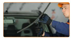
Remove the blade from the wiper arm.
