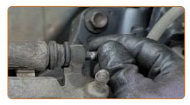
Tighten the brake caliper fasteners. Use a drive socket #14. Use a torque wrench. Tighten it to 32 Nm torque.
