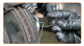
Remove the brake pads. Use a crowbar.
