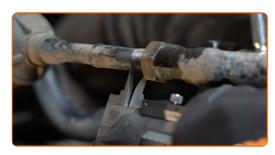
Loosen the lock nut securing the tie rod end to the tie rod. Use a combination spanner #22.
