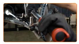
Tighten the tie rod end locknut. Use a combination spanner #19. Use a combination spanner #22. Use a torque wrench. Tighten it to 88 nm torque.
